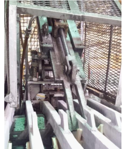
Picture 8. Mechanism to tilt the plastic piece
