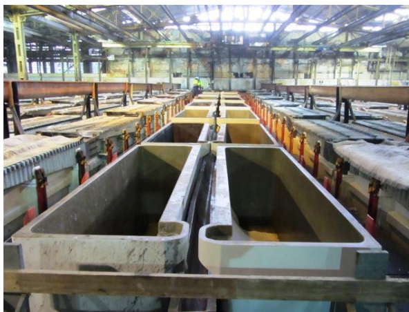
Picture 1 Polymeric concrete electrolytic cells
