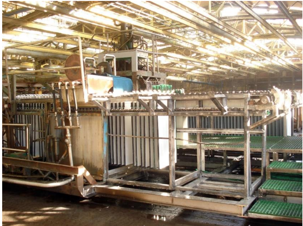
Picture 11. Cathode Outlet Conveyor
