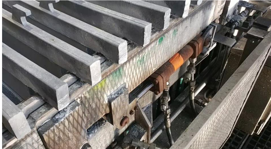
Picture 15. Hydraulic Walking Beams
